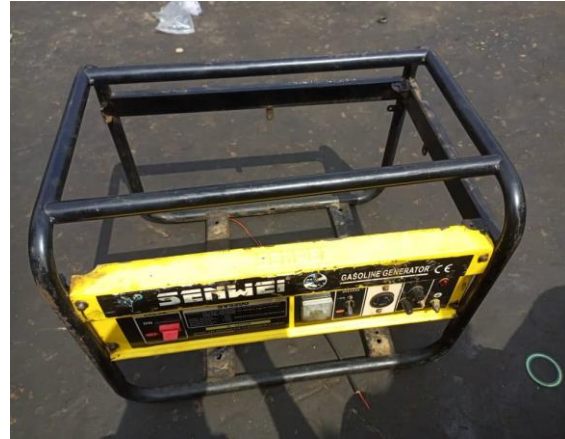
Figure 4. Metal base frame.
